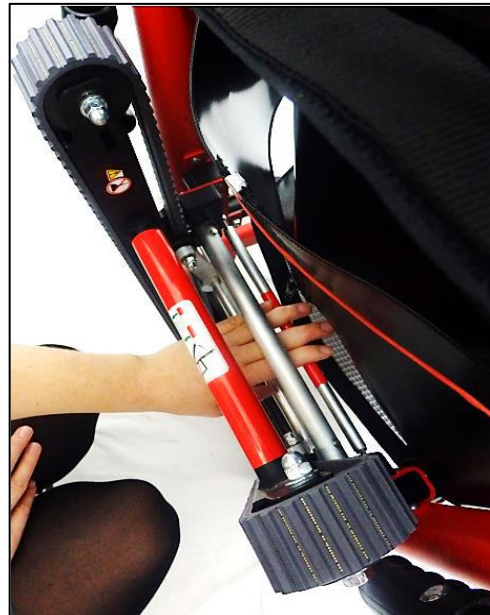
Releasing Track from push-to-close latches
