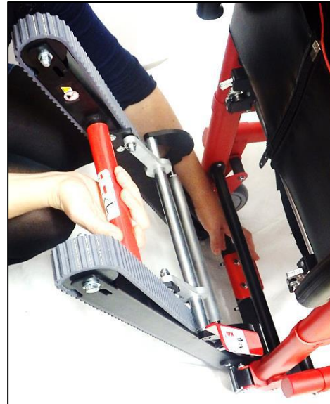
Locating lower Track lock onto axle
