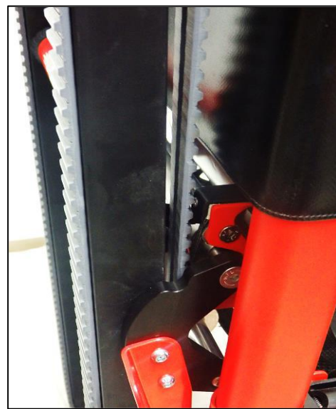
Track attached to Chair back via push-to-close latches
