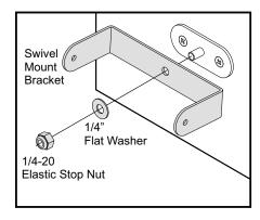
Secure the Control Head/Adapter Plate assembly onto the swivel mount bracket as shown and secure using the hardware provided.
