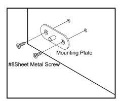
Secure the Swivel Mount Bracket to the mounting plate as shown using the hardware provided.
